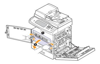
Pull the used imaging unit out of the machine using the handle on its bottom.
